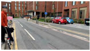
Figure 63. Existing modal filter on Walnut Tree Close allows northbound through traffic and restricts southbound through traffic. Cyclists are permitted bi-directionally. Proposal to restrict all through traffic and allow access only.
